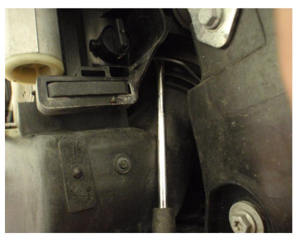
11. On the drivers side of the intercooler ,depress the clip holding the intercooler to the car with a flat bladed screwdriver. At the same time ,push the intercooler to the left (looking from the front of the car ) to release from the bracket on the passenger side , then pull down to release the passenger side connector.
