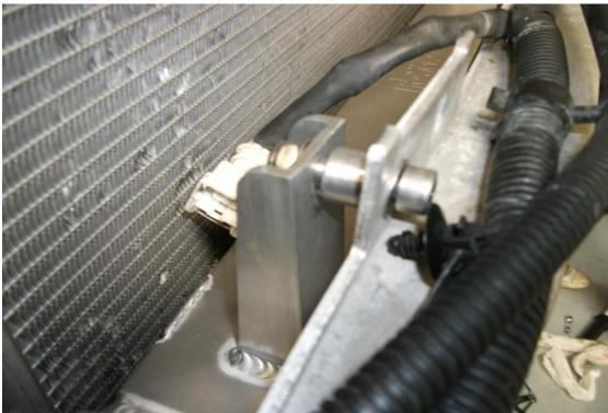
14. Push the passenger side into the hose first, until you hear a click signifying that the retaining wire clip is seated correctly in the recess of the connector . Make sure that the bracket shown below is on the OUTSIDE of the plastic attached to the car.
