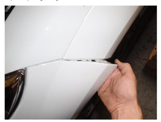
6. Lift the bumper forwards slightly off the car ,until you can access the electrical connector on the inside of the bumper passenger side (RHD)or drivers side on (LHD). Ensure the ignition is of and detach the harness
