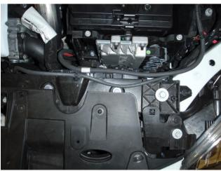
4. Undo the  $\sin T20$  screws on the top of the bumper .
