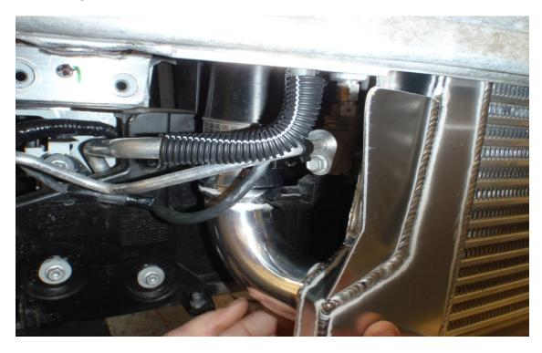
15. Now tighten the two m8 x 30 allen caps from step 13 using a 6mm allen key and 13 mm spanner.
