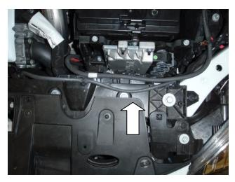
Pull the airfeed upwards to release it from the top of the bumper, then pull the front section of the battery cover to release it from the battery
